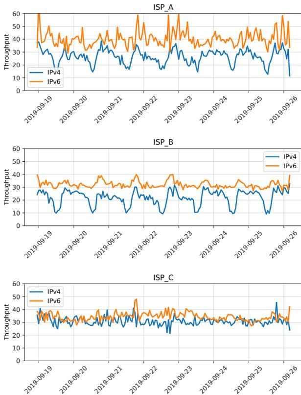
**Figure 9: IPv4 and IPv6 throughput (Mbps) for the three major ISPs of Section 4.**
